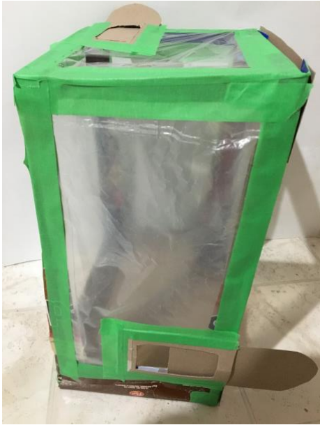
13. Fabricate and install a second ventilation gate at the bottom corner, opposite from the ventilation gate on the roof.
