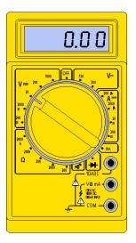
Generally multimeters have a central knob with various positions to which it can be rotated. Where you position the knob will be dependent on the purpose for which you will use it. If you circuit is operating from a constant voltage source such as a battery, current flow will always be in the same direction, and thus it is
