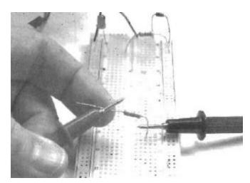
You should not hold the both sides of the wire or component while you are testing the resistance, because your skin will conduct electricity and the DMM will be measuring your resistance mixed with the component's.
