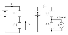
In order to measure voltage across a given component in your circuit, the voltmeter is connected *in parallel* to that component. Because the voltmeter provides a parallel pathway, it should pass as little current as possible, so as not to short circuit the component across which it is measuring. That being said, a voltmeter should have *very high* resistance.
