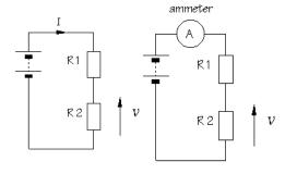
To measure current, the multimeter should be connected *in series* with the rest of the components in your circuit. This allows the current flowing through the circuit to pass through the ammeter as well. However, meters should not alter the behavior of the circuit whose current they are measuring, and thus, to avoid causing a voltage drop across them, ammeter should have *very low* resistance.
