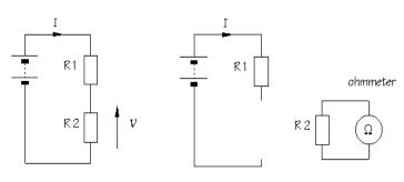
Unlike ammeters and voltmeters, ohmmeters cannot function if the circuit is connected to a power supply. In order to measure the resistance of a given circuit component, it must be <u>removed</u> from the circuit and probed independently. The ohmmeter then passes a small current through the circuit component of interest and subsequently measures the voltage produced, and using principles based on Ohm's law,
