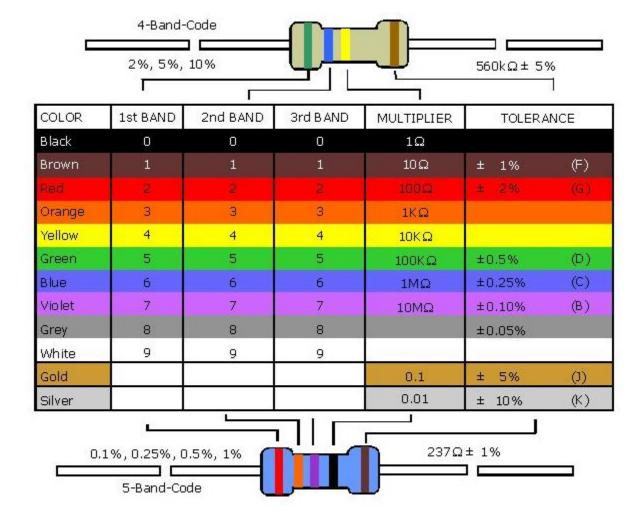
For example, a resistor with color code **red**, **violet**, **yellow gold** is a resistor with a value of 270k  $\Omega$  and a 5% tolerance. Thus the actual value of the resistor is between 256.5k $\Omega$  and 283.5k $\Omega$ . More expensive resistors have lower tolerance.
