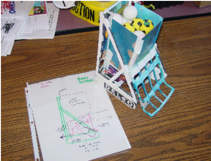
Competition robot sketch and mock-up to validate a design (Image from TechnoKats)
