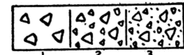
• STAGES IN MAKING CONCRETE SYMBOL •
