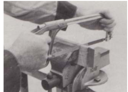
The correct method of holding a hand hacksaw – courtesy Kostel Enterprises Ltd.
