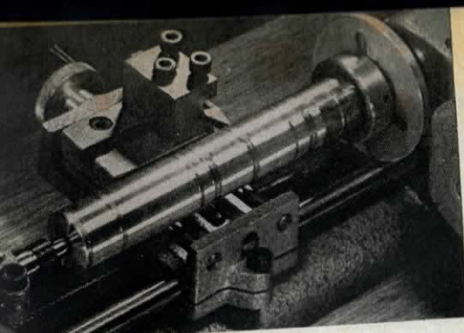
BARREL BLANK , mounted between centers, is driven by special faceplate dog made from ball-bearing ring
