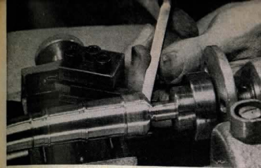
HAND-HELD CHISEL resting on blank bit clamped in toolholder is used to shape final breech contours
