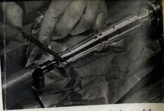
AFTER RIDGES are machined square they're rounded with Swiss-type file as done here at gun's muzzle end
