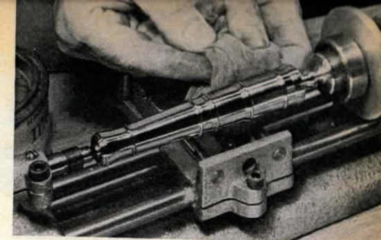
COMPLETED BARREL is polished in the lathe with a brass polish; the ball end is hand-finished later
